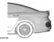
The system uses radar sensors that are located behind the bumper fascia on each side of your vehicle. Do not allow mud, snow or bumper stickers to obstruct these areas, this can cause degraded system performance. See **Blind Spot**Information System (page 232). If the Blind Spot Information System is blocked, Cross Traffic Alert is also blocked. A corresponding message appears in the information display as soon as you shift
