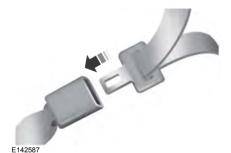
Insert the belt tongue into the proper buckle (the buckle closest to the direction the tongue is coming from) until you hear a snap and feel it latch. Make sure you securely fasten the tongue in the buckle.
