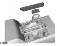
Locate the white brake shift interlock lever on the passenger side of the shifter assembly.
