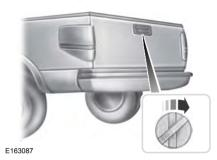
Insert the ignition key into the tailgate lock. Turn it clockwise to lock the tailgate. Turn it counterclockwise to unlock the tailgate.
