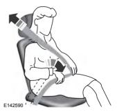
Pregnant women should always wear their safety belt. Position the lap belt portion of a combination lap and shoulder belt low across the hips below the belly and worn as tight as comfort will allow. Position the shoulder belt to cross the middle of the shoulder and the center of the chest.
