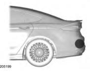
The system uses radar sensors that are located behind the bumper fascia on each side of your vehicle. Any dirt, mud and snow in front of the sensors and/or driving in heavy rain can cause system degradation. Also, other types of obstructions in front of the sensor can cause system degradation. This is referred to as a 'blocked' condition.
