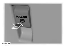
You can release the electric parking brake either manually by pressing the switch or automatically.
