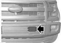
A message displays if something obstructs the radar signals from the sensor. The sensor is behind a cover near the driver side of the lower grille. The system cannot detect a vehicle ahead and does not function when something obstructs the radar signals. The following table lists possible causes and actions for this message displaying.
