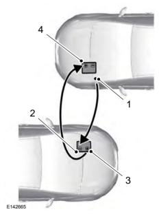
1. Remove the negative (-) jumper cable from the disabled vehicle.
