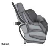
3. While holding both shoulder and lap portions next to the tongue, route the tongue and webbing through the child seat according to the child seat manufacturer's instructions. Be sure that the belt webbing is not twisted.
