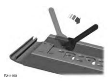
Note: A smooth surface tool can be used to rotate the stops.
