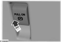
Pull the switch up to apply the electric parking brake.
