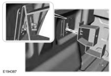
Hook the top of the ramp holder over the mounting plate and rotate the ramp holder into position.
