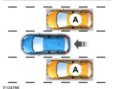
The Blind Spot Information System is designed to aid you in detecting vehicles that may have entered the blind spot zone (A). The detection area is on both sides of your vehicle, extending rearward from the exterior mirrors to approximately 13 ft (4 m) beyond the bumper. The system is designed to alert you if certain vehicles enter the blind spot zone while driving.
