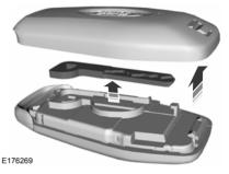
Slide the release on the back of the remote control and pivot the cover off to access the key blade.
