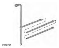
Use your key to remove the lock cylinder from the access hole of the bumper to allow access to the guide tube. Assemble the jack handle as shown in the illustration.
