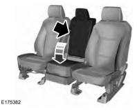
Press the release control to move the front seat armrest up or down.
