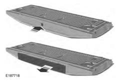
3. Pull the step out fully. Lower the step to its lowest position.
