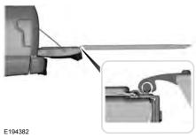
5. Slide the ramp claw onto the tailgate plate.
