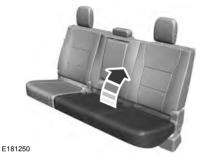
Rotate the seat cushion up until it locks into the vertical storage position.
