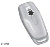
1. Slide the release on the back of the remote control and pivot the cover off.
