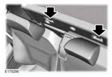
If the tether strap is clipped incorrectly, the child safety seat may not be retained properly in the event of a crash.
