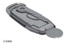
2. Insert a coin into the slot and twist to separate the housing.
